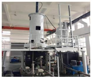
Figure 7. Preparing and breaking system of the hydrate
