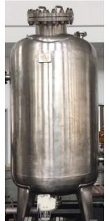
Figure 10. Efficient three-phase separator
