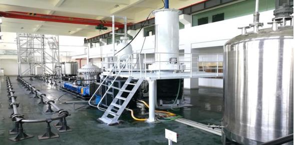
Figure 6. The process of marine natural gas hydrate solid fluidization exploitation experimental system
