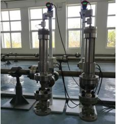
Figure 11. Real-time phase content monitoring sampler
