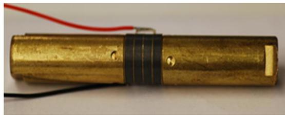
**Figure 1.** A typical Langevin transducer.
