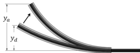
**Figure 4.** Composite actuator in its deactivated ( $y_d$ ) and activated ( $y_a$ ) states.
