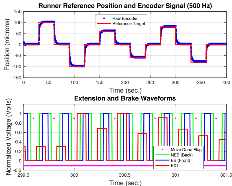
Figure 6. Simulated step responses of the 20-micron FIA. The top subplot shows the simulated position command and encoder signal. The bottom subplot shows a closeup of the brake and extension waveforms at 300 s. Note the two multiple step moves just after the position command is changed.
