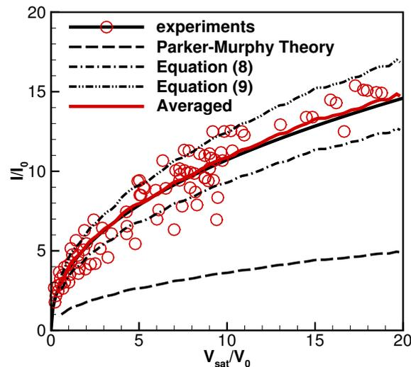
**Figure 5.** Comparisons of current-voltage results. Symbols: measurements in space mission (solid black line: the best fitting curve); Long dashed line: P-M theory; Black dash-dot lines: new enhancement factors (solid red line: their average).
