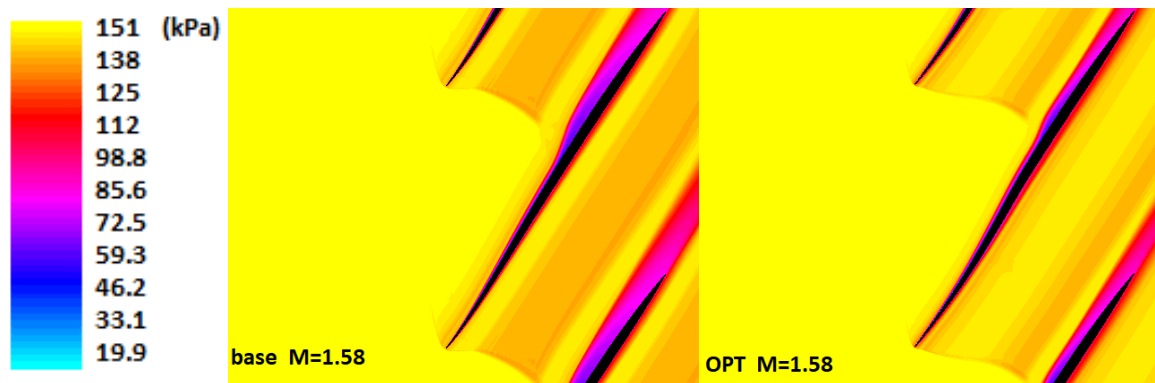
Figure 16. Total pressure contours (kPa) of optimized profile at Mach 1.58.
