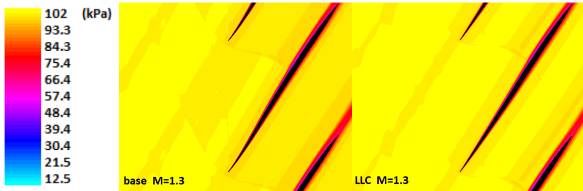
Figure 14. Total pressure contours (kPa) of profiles with LLC at Mach 1.3.
