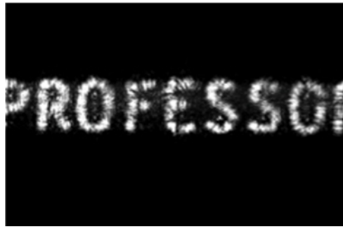
Figure 3. Input object captured by camera. Here the slide with the word “PROFESSOR” is placed directly to the detector. The size of the object slightly exceeds the size of the detector.
