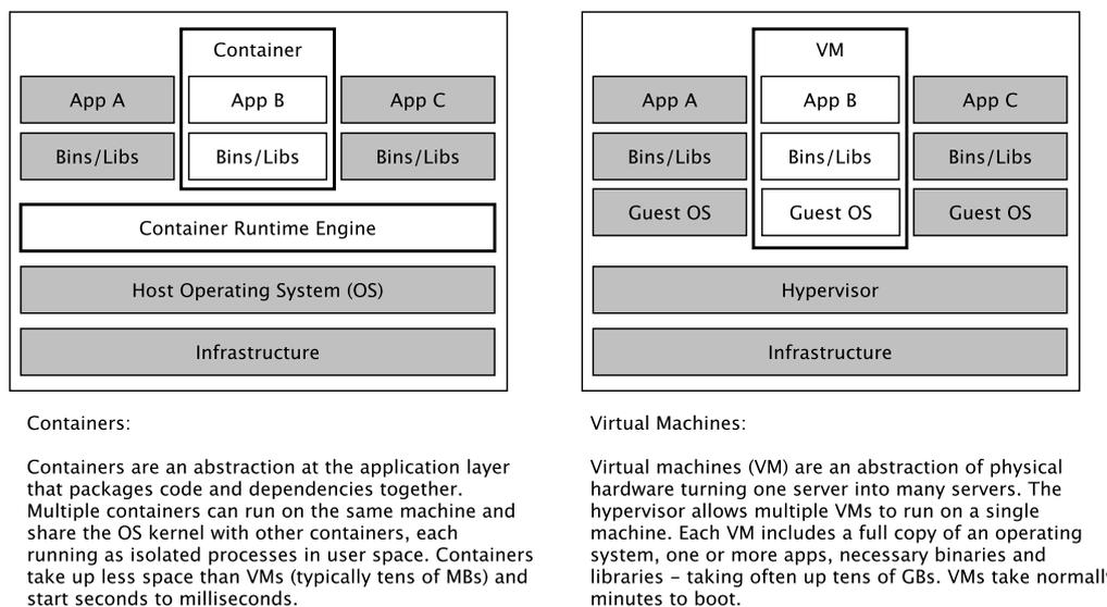
Figure 5. Comparing containers and virtual machines (adapted from the Docker website).
