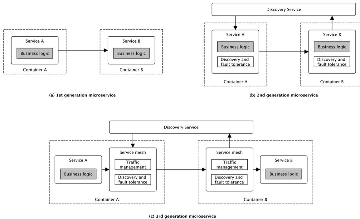
Figure 7. Microservice architecture evolution—adapted from [31].
