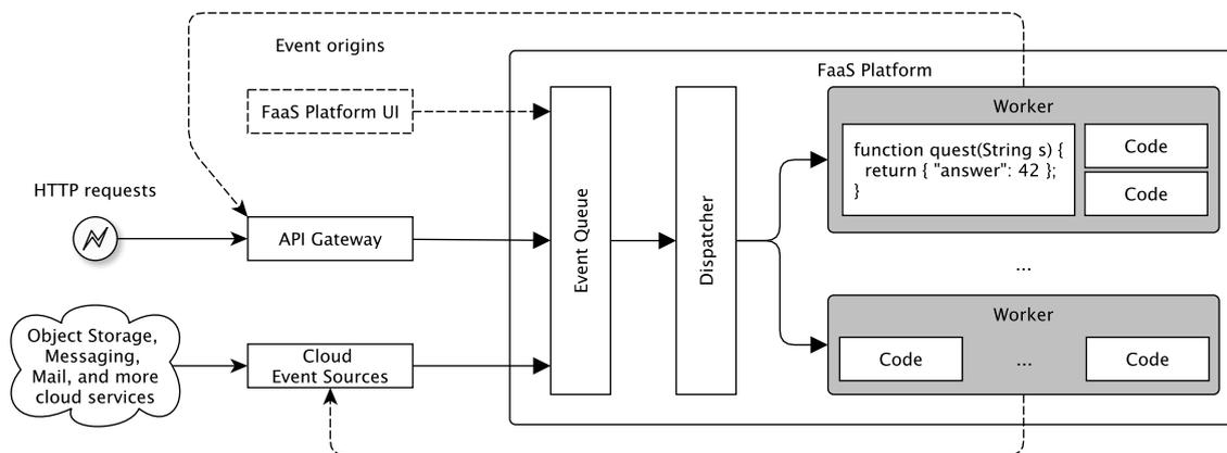
Figure 8. Blueprint of a serverless platform architecture (adapted from [42]).
