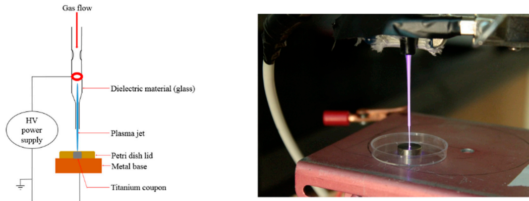
Figure 2. Schematic diagram and photograph of the jet plasma setup. The figure on the left demonstrates the schematic diagram of the jet plasma and the photograph on the right shows the actual experimental setup of jet plasma treating the Ti coupon (12.7 mm diameter and 3 mm thickness).
