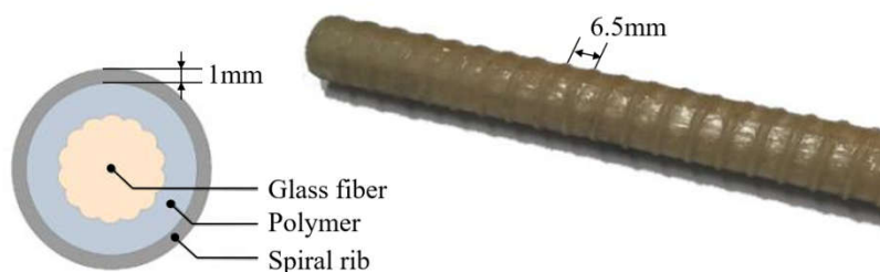
Figure 3. Surface aspect of the glass fiber reinforced polymer (GFRP) bar.
