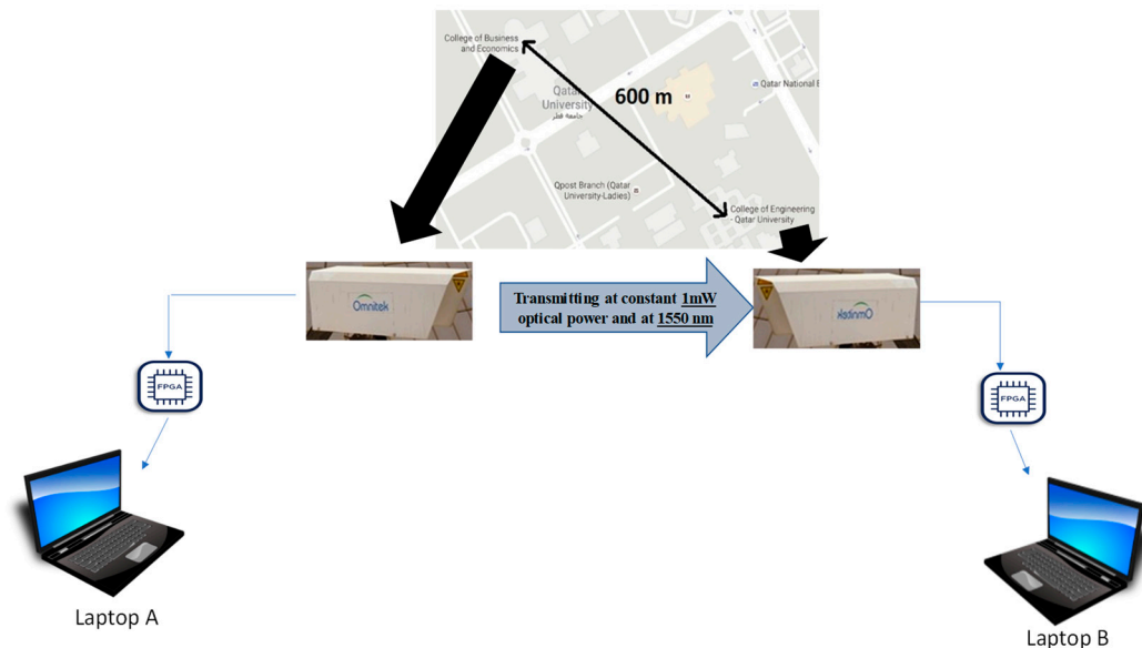
Figure 1. Details of the free-space optical (FSO) system installed at Qatar University.
