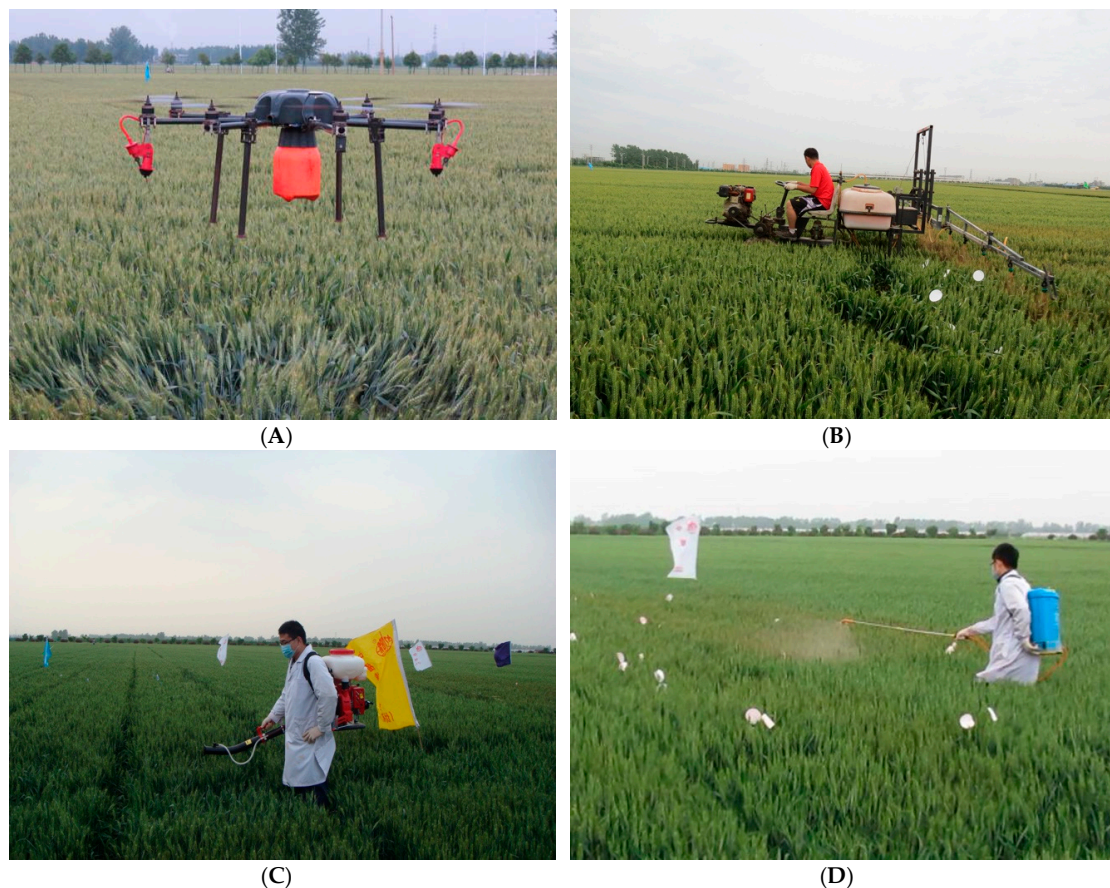
Figure 1. Four test sprayers: (A) 3WTXC8-5 six-rotor unmanned aerial vehicle (UAV) sprayer; (B) 3WX-280H self-propelled boom (SPB) sprayer; (C) WFB-18 knapsack mist-blower (KMB) sprayer; and (D) 3WBS-16A2 electric air-pressure knapsack (EAP) sprayer.
