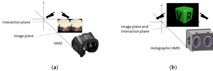
Figure 5. (a) Image plane and convergence plane of the stereoscopic display. (b) Image plane and convergence plane of the holographic display (the convergence plane is the same as the interaction plane). HMD, head-mounted display.
