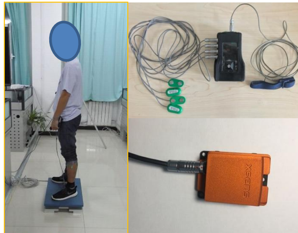
Figure 4. Upright standing push-recovery. Left picture shows a subject standing on the force plate. Pushing force is exerted on his back. Right upper picture shows the sEMG device. Right lower picture shows the IMU sensor.
