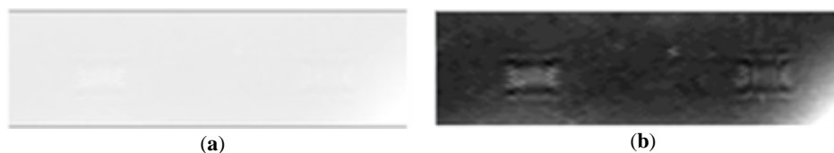
Figure 19. The (a) original and (b) enhanced images of notches 1 and 2 under the 4 mm-thick rubber layer, obtained at a standoff distance of 0.1 mm.
