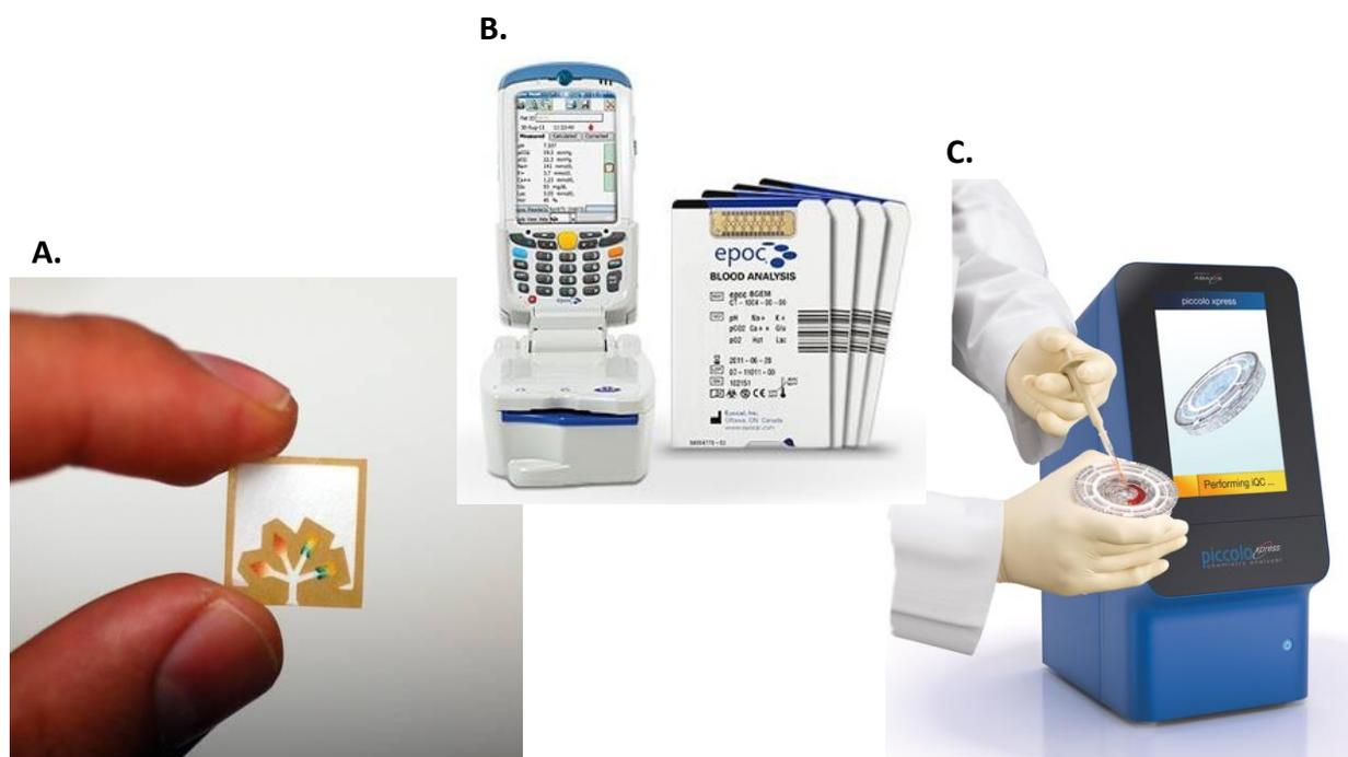
**Figure 3.** Examples of microfluidic-based platforms. (A) Paper-based microfluidic device for simultaneous quantification of glucose and other analyte in urine. Taken from <http://gmwgroup.harvard.edu> with permission from Prof. Whitesides; (B) Lab-on-a-chip platform developed by Alere for blood chemistry analysis. Reproduced with permission from Alere; (C) Lab-on-a-disc diagnostic device designed by Abaxis. Reproduced with permission from Abaxis.
