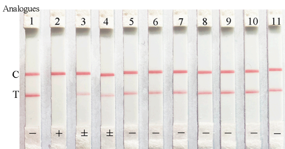
Figure 5. The cross-reactivity tests of the ICA for ZEN detection. The analogs were 5 ng/mL. (1) negative; (2) ZEN; (3) \alpha -Zearalenol; (4) \beta -Zearalenol; (5) \alpha -Zearalanol; (6) \beta -Zearalanol; (7) Zeranol; (8) Aflatoxin B 1 ; (9) Deoxynivalenol; (10) Fumonisin B 1 ; (11) Ochratoxin A.
