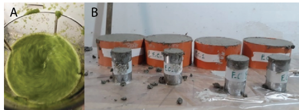
Figure 3. Centrifugation of fennel side-products (A) and preparation of cylindrical bricks for acoustic tests (B).
