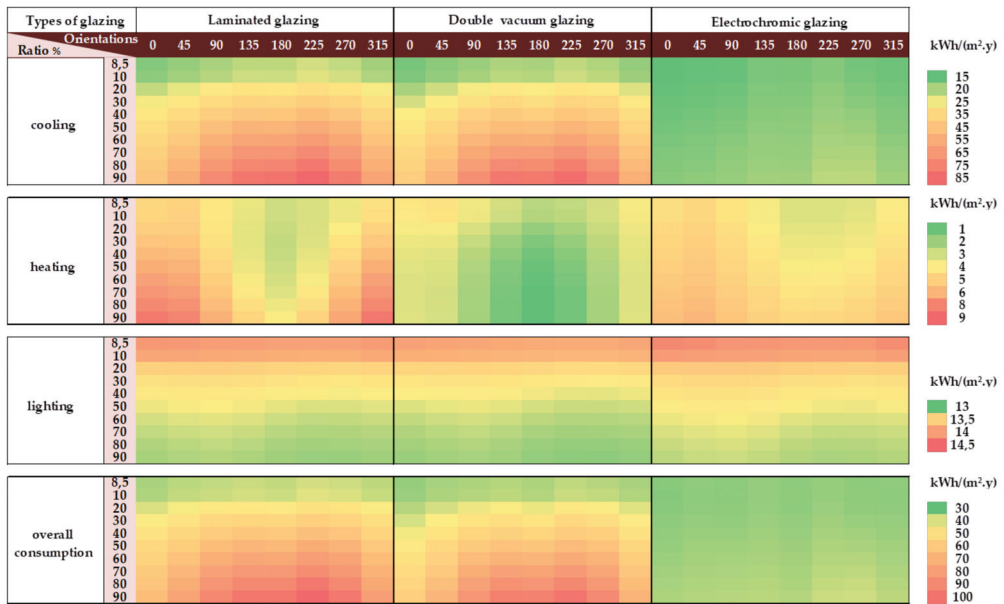
Figure 4. Energy consumption as a function of WWR, glazing window, and orientation for Cooling. Heating. Lighting. Overall consumption.
