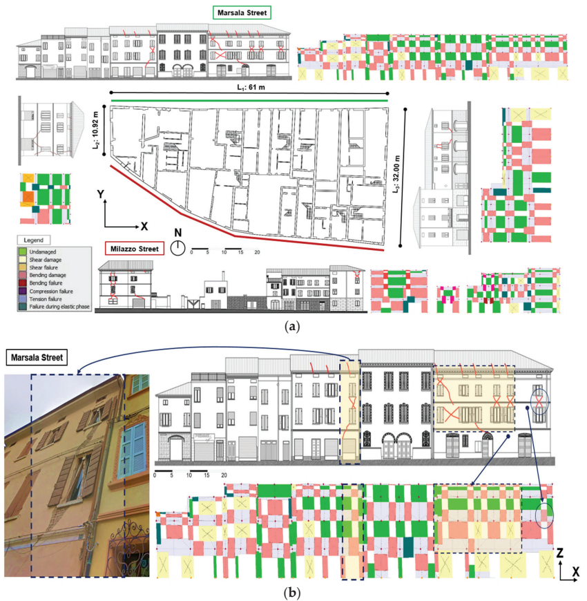
Figure 10. Validation of the mechanical model by comparison between real damages and numerical ones (a,b).
