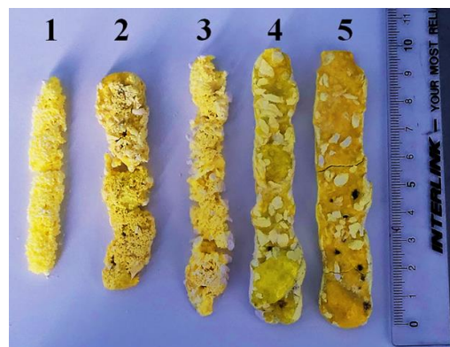
Figure 4. Photographs of YAG:Ce ceramic samples synthesized under the influence of electron fluxes of different E and P : 1— E = 1.4 MeV, P = 2.5 kW/cm 2 ; 2— E = 2.0 MeV, P = 4 kW/cm 2 ; 3— E = 2.5 MeV, P = 8 kW/cm 2 ; 4— E = 2.0 MeV, P = 6 kW/cm 2 ; 5— E = 2.5 MeV, P = 10 kW/cm 2 .
