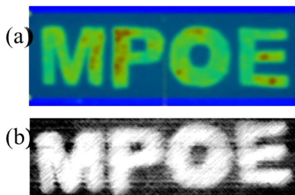
Figure 8. (a) Persistent luminescence image from the “MPOE” pattern, hand painted using ZGSO-3: \text{Ni}^{2+} , \text{Er}^{3+} , \text{Cr}^{3+} NPs detected with Si-based visible camera; (b) persistent luminescence image from the “MPOE” pattern, hand painted using ZGSO-3: \text{Ni}^{2+} , \text{Er}^{3+} , \text{Cr}^{3+} NPs, detected with InGaAs-based NIR camera.
