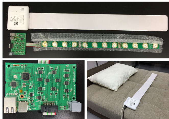
Figure 3. The sleep monitoring sensor used in the study is mainly composed of 12 piezoelectric sensors as the upper image and a control circuit with LAN communication functionality as the bottom left image. The scenario of sleep monitoring sensor being placed on a bed is shown in the bottom right image.
