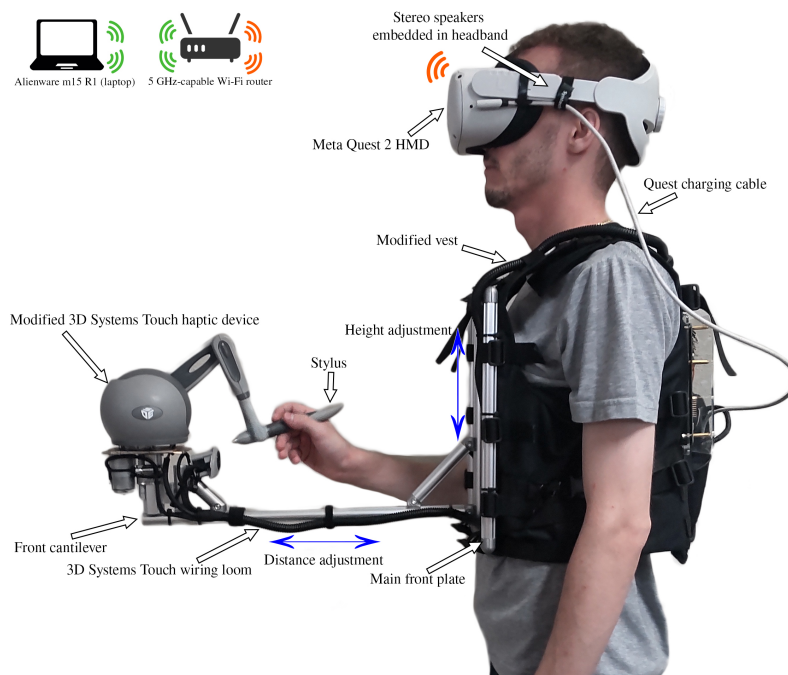
Figure 2. System assembly profile depicting the wearable harness and its adjustability, supporting the devices used for personal sensing. Head-mounted display (Meta Quest 2) and modified haptic force-feedback stylus (3D Systems Touch).
