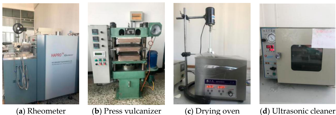
Figure 1. Main experimental equipment.
