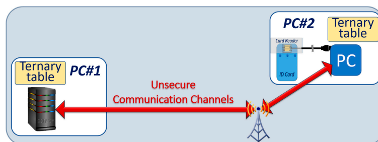
Figure 8. Block diagram of the experimental set up to study the public key distribution with ternary tables. The tables are stored in the server, and in the smartcard.
