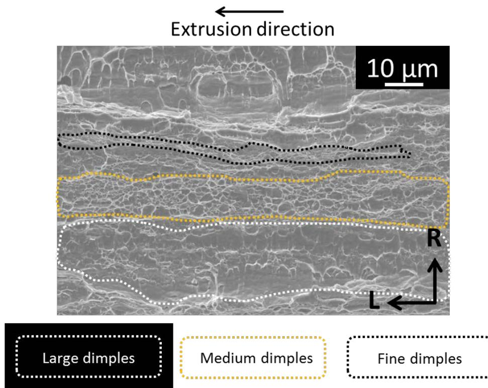
*Fig. 1 SEM fracture surface image of ODS-KIT HE at  $200 \text{ }^\circ\text{C}$  in the C-R orientation. Three different zones of dimples with different sizes are observed.*
