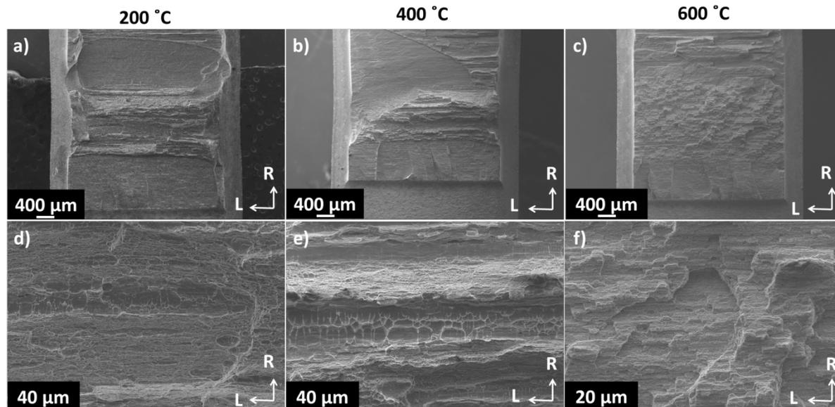
Fig. 2 Fracture surfaces of the C-R oriented specimens at 200 °C (a and d), 400 °C (b and e) and 600 °C (c and f) of ODS-KIT HE.
