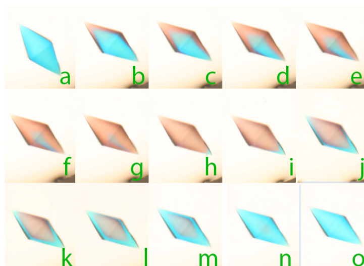
Figure 10. A tetragonal crystal of thaumatin was saturated with the copper porphyrin dye Luxol blue (Solvent blue 38) in (a) and dithionite then added to the mother liquor (b). The blue color transitioned to elemental copper as the dye was reduced. At about (k) oxygen from the environment began to re-oxidize the copper to the \text{Cu}^{2+} state and the dye regained its blue color. In both the reduction and oxidation phases the redox front was well defined. The series of images (a–o), taken at appropriate time intervals, shows the progress of the dye.
