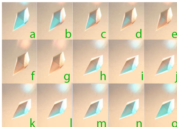
Figure 9. A tetragonal crystal of thaumatin about 1 mm in length was saturated with the redox sensitive dye Luxol blue (Solvent blue 38) giving it an intense blue color. Luxol blue is a porphyrin that contains a copper ion in the plus two state that is responsible for the color. Solid dithionite was added directly to the mother liquor, which reduced the \text{Cu}^{2+} ion to elemental copper. Thus, the transformation of color in the crystal from blue to copper shows the progress of the reduction reaction as the dithionite penetrated the crystal. Beginning with image (h), oxygen in the environment initiated re-oxidation of the copper and the color transitioned again to blue. This is shown in the final images (i) through (o). The series of images (a–o), taken at appropriate time intervals, shows the progress of the dye.
