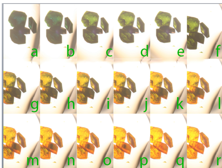
Figure 5. Tetragonal lysozyme crystals saturated with the dye bromocresol green are a dark blue-green color at pH 6.0 in (a). When the pH of the mother liquor was altered to pH 3.8, the crystals were seen in (b) through (r) to change in color to yellow. The series of images (a–r), taken at appropriate time intervals, shows the progress of the dye.
