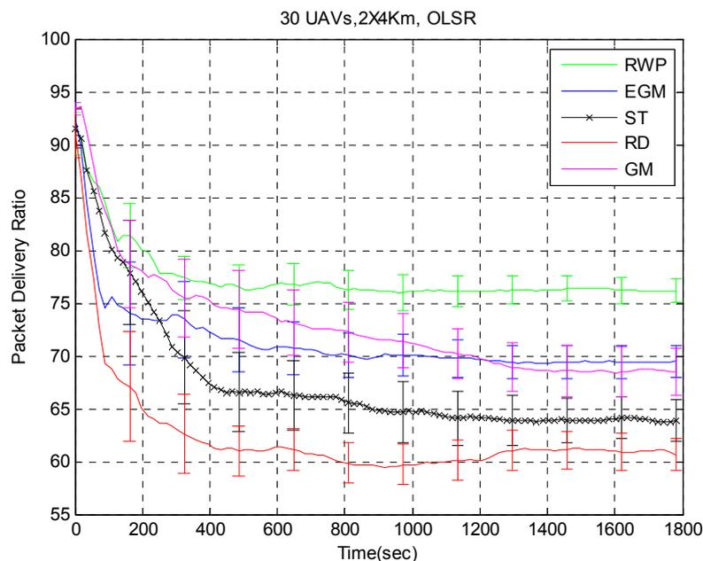
Figure 15. PDR of optimized link state routing (OLSR) under various mobility models.
