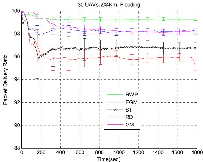
**Figure 17.** PDR of flooding under various mobility models.
