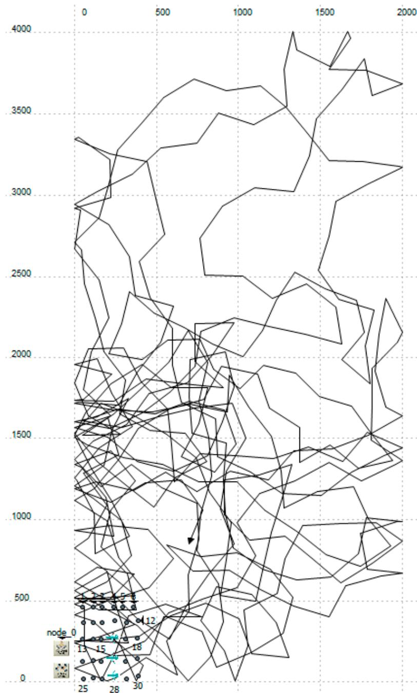
**Figure 4.** Trajectory of a UAV under the Gauss–Markov (GM) model.
