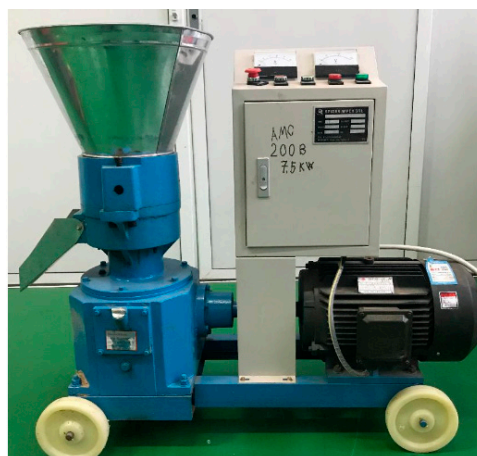
Figure 3. Pelletizer used for pellets production.
