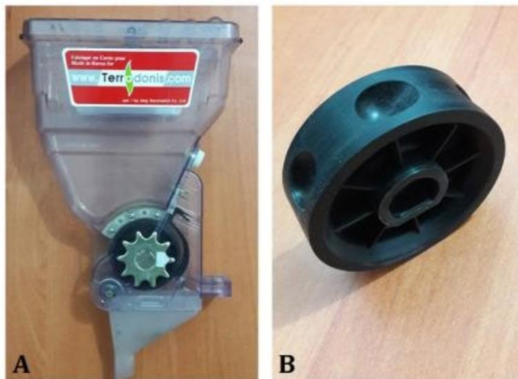
**Figure 14.** The Terradonis celled roller seed meter system - A) The complete seed meter unit, B) one of the provided celled rollers
