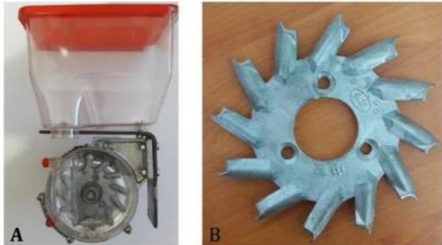
**Figure 9.** Finger vertical plate seed meter system - A) Seed unit with seed container and seed meter system, B) aluminum vertical seed plate
