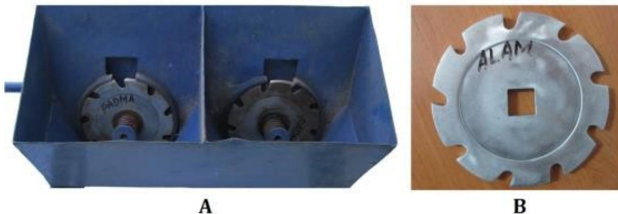
**Figure 7.** The BARI -9-cell inclined plate seed meter - A) Frame with two seed meter units, B) aluminum seed plate
