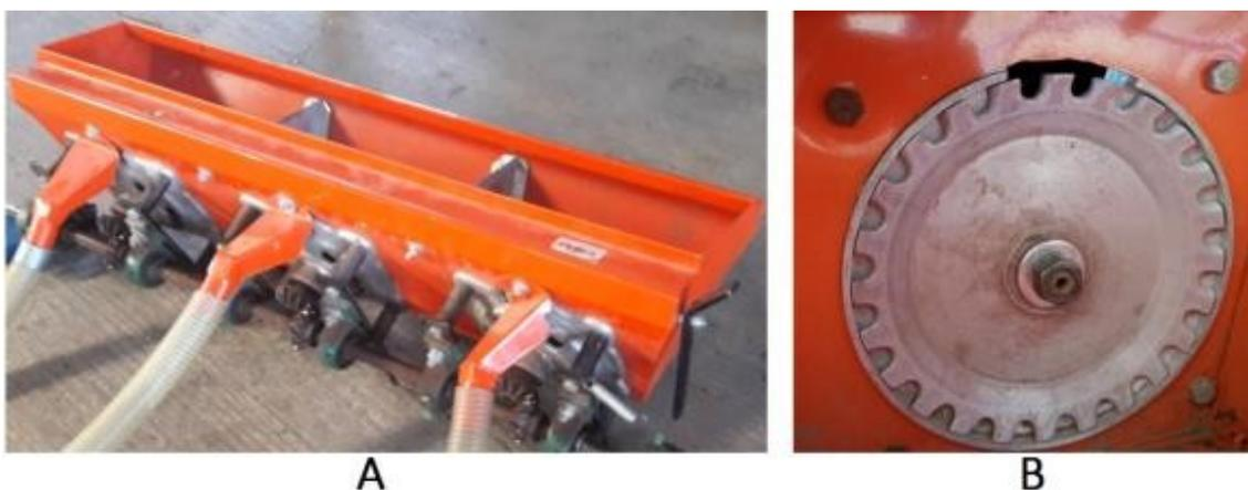
**Figure 6.** Sembradoras TIMS inclined plate seed meter - A) Single seed unit with 3 seed sections, B) aluminum 24-cell seed plate
