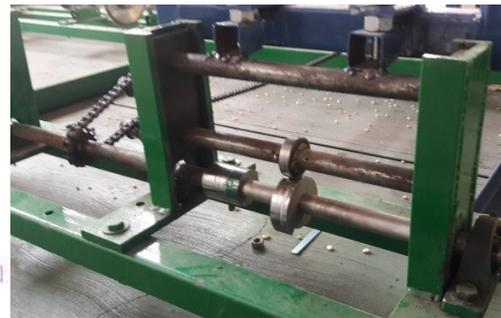
**Figure 3.** Schematic of the vibration generation mechanism of the test-bench (left) and detailed view of the shell-shaped cam shaft (right)
