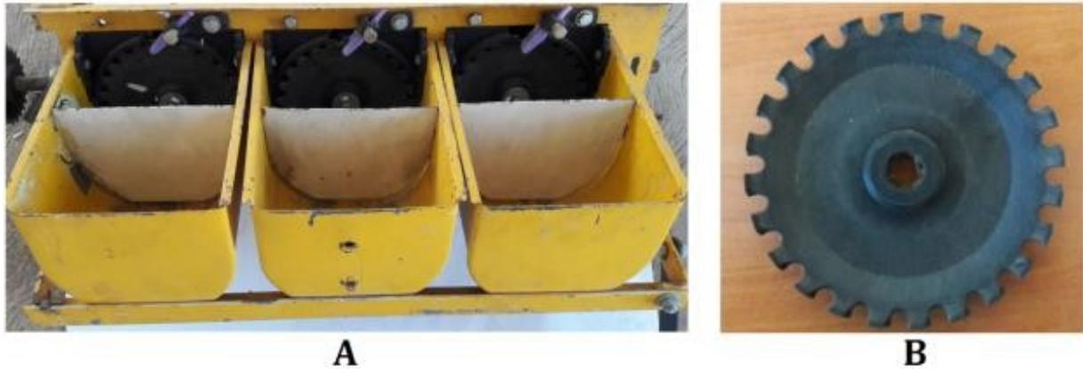
**Figure 4.** The National Agro Industries inclined plate seed meter - A) a modular setup of 3 inclined plate seed meter units, B) 24-cell seed plate
