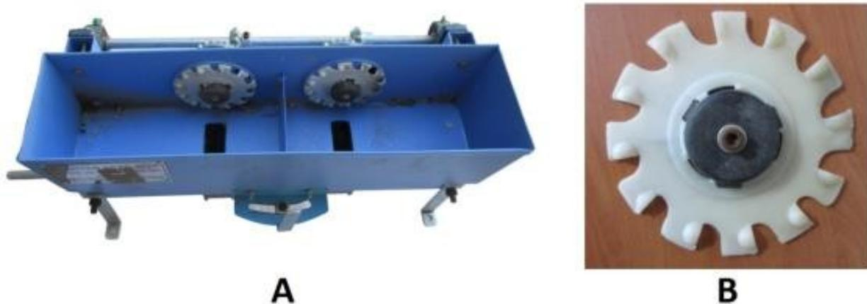
**Figure 8.** VMP-12 vertical plate seed meter – A) Frame with two seed meter units, B) Plastic bucket or spoon-like vertical plate
