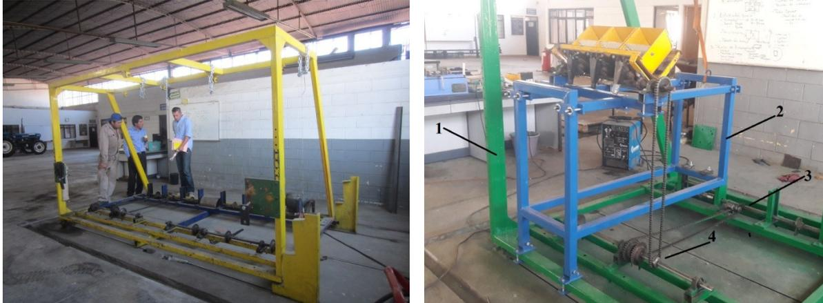
**Figure 2.** Bridge set up at CENEMA with steps for adding an angle to the structure (left) and a set of 3 seed meters mounted on a fixed frame during the trials with 1) the supporting bridge, 2) the mounted frame, 3) the vibration cam shaft and 4) the chain transmission (right)
