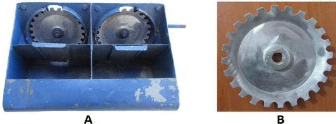
**Figure 5.** The BARI 24-cell inclined plate seed meter - A) Seed meter unit with container and central divider gate, B) aluminum 24-cell seed plate
