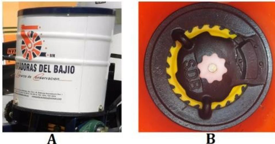
**Figure 11.** Sembradoras del Bajío horizontal Plate Seed meter system - A) Seed container, B) Horizontal plate and ejection chamber
