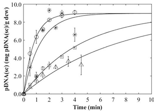
**Figure 6.** Kinetics of pDNA(sc) release with a mill frequency of 15 Hz. (o) Experiment 1:  $k = 1.24 \text{ min}^{-1}$ ; (\*) Experiment 3:  $k = 0.76 \text{ min}^{-1}$ ; ( $\Delta$ ) Experiment 5:  $k = 0.14 \text{ min}^{-1}$ ; ( $\square$ ) Experiment 7:  $k = 0.22 \text{ min}^{-1}$ ; (—) model fit. Data represent the means of two replicates and error bars represent the standard deviation.
