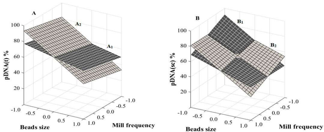
**Figure 4.** Response surface plots. (A) Effect of mill frequency and bead size in the release of pDNA(t). (A<sub>1</sub>) Low cell concentration (10 g wcv/L) and (A<sub>2</sub>) high cell concentration (20 g wcv/L). (B) Effect of mill frequency and bead size in the release of pDNA(sc). (B<sub>1</sub>) Low cell concentration (10 g wcv/L) and (B<sub>2</sub>) high cell concentration (20 g wcv/L).
