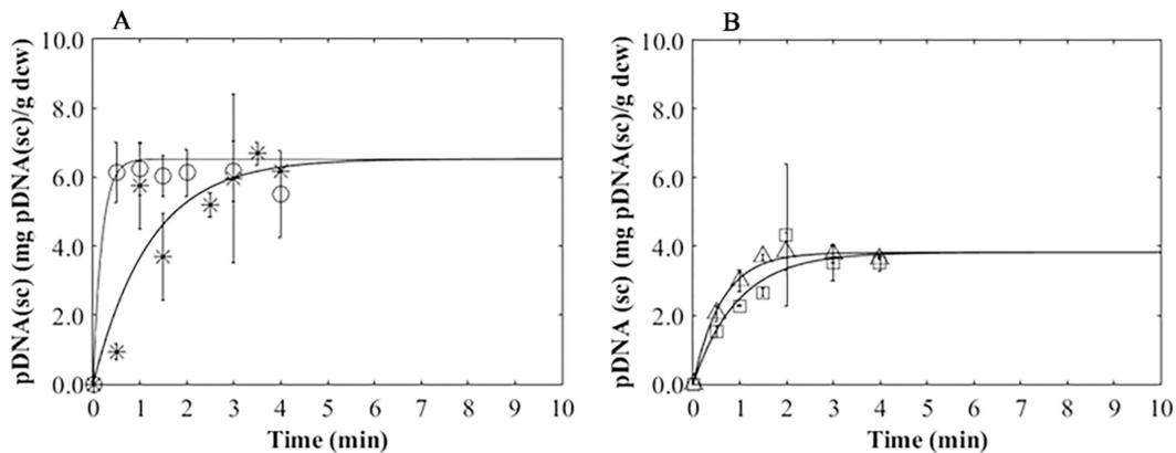
**Figure 7.** Kinetics of pDNA(sc) release with a mill frequency of 30 Hz. (A) (o) Experiment 2:  $k = 5.40 \text{ min}^{-1}$ ; (\*) Experiment 4:  $k = 0.82 \text{ min}^{-1}$ . (B) ( $\Delta$ ) Experiment 6:  $k = 1.62 \text{ min}^{-1}$ ; ( $\square$ ) Experiment 8:  $k = 1.04 \text{ min}^{-1}$ ; (—) model fit. Data represent the means of two replicates and error bars represent the standard deviation.
