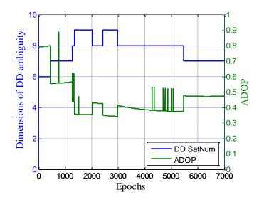
Figure 11. Visible DD satellite number and ADOP value.
