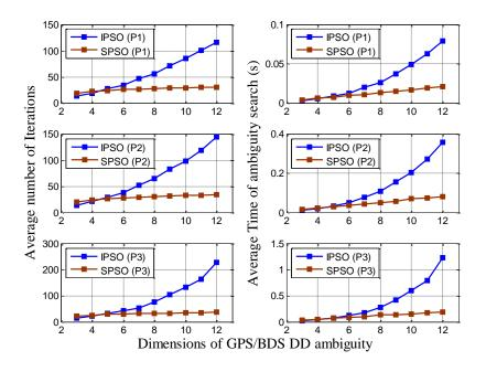
**Figure 7.** Average number of iterations and search time of IPSO/SPSO–AR under various DD ambiguity dimensions in Scheme #2.
