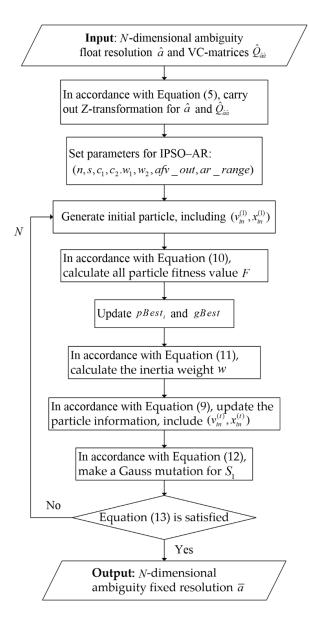
**Figure 1.** Flow diagram of IPSO–AR (improved particle swarm optimization–ambiguity resolution). VC: variance–covariance matrix.
