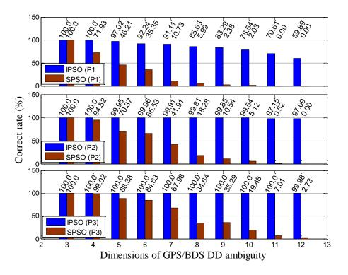
Figure 8. Correct rates of IPSO/SPSO-AR under various DD ambiguity dimensions in Scheme #2.
