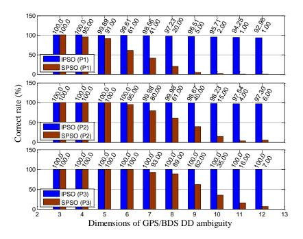
Figure 6. Correct rates of IPSO/SPSO-AR under various DD ambiguity dimensions in Scheme #1.
