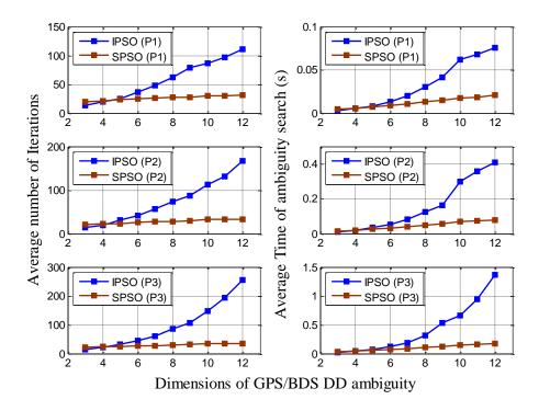
**Figure 9.** Average number of iterations and search time of IPSO/SPSO–AR under various DD ambiguity dimensions in Scheme #3.
