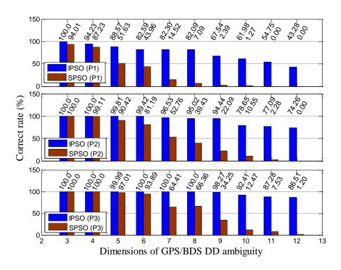
Figure 10. Correct rates of IPSO/SPSO-AR under various DD ambiguity dimensions in Scheme #3.
