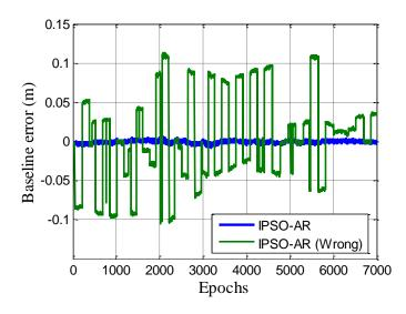
**Figure 13.** Baseline length errors after single-epoch real-time kinematic (RTK) process with IPSO–AR method.
