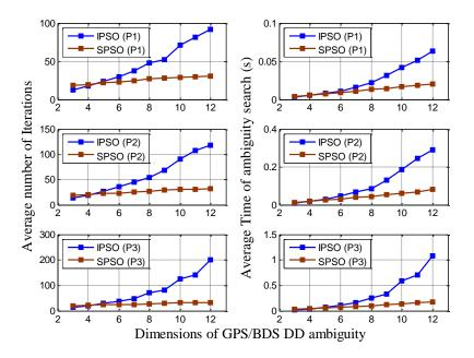
**Figure 5.** Average number of iterations and search time with various DD ambiguity dimensions for IPSO/standard PSO algorithm (SPSO)–AR under Scheme #1. GPS: Global Positioning System; BDS: BeiDou Navigation Satellite System.
