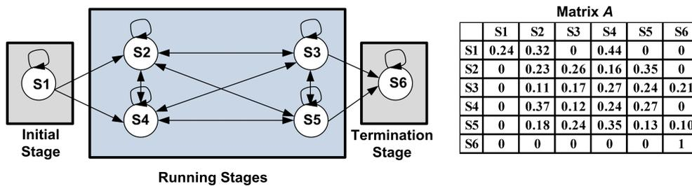
Figure 3. A six-state program behavior-aware HMM topology and its corresponding transition probability matrix  $A$ .
