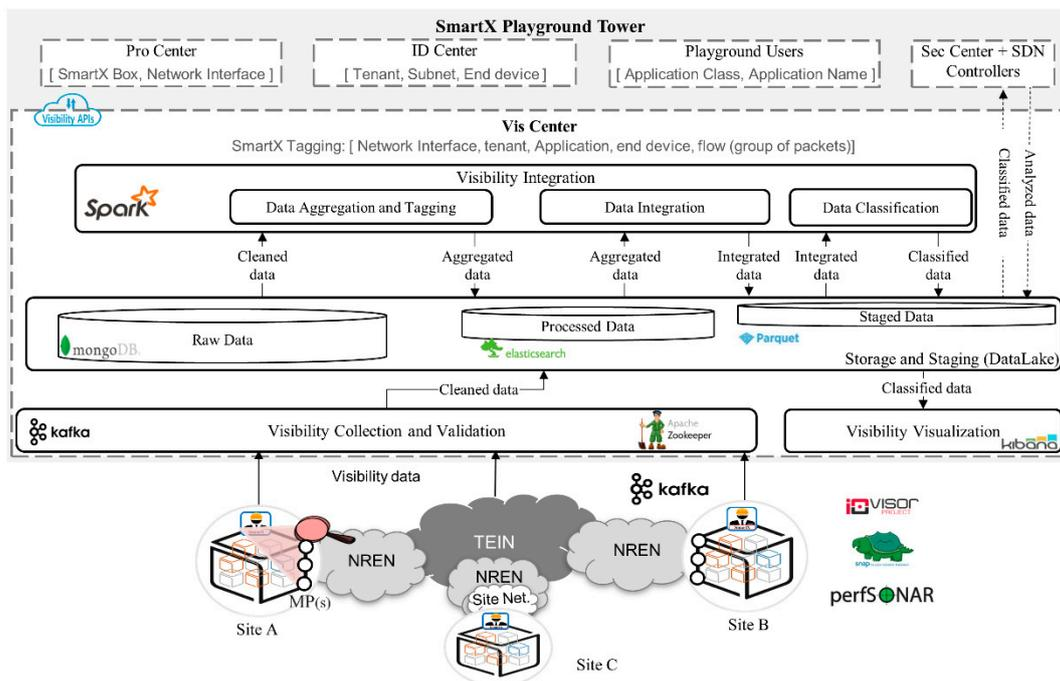
Figure 3. The overall architecture of SmartX MVF with the extension of flow-centric visibility.
