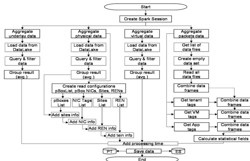
Figure 6. Design of visibility data aggregation and tagging component.
