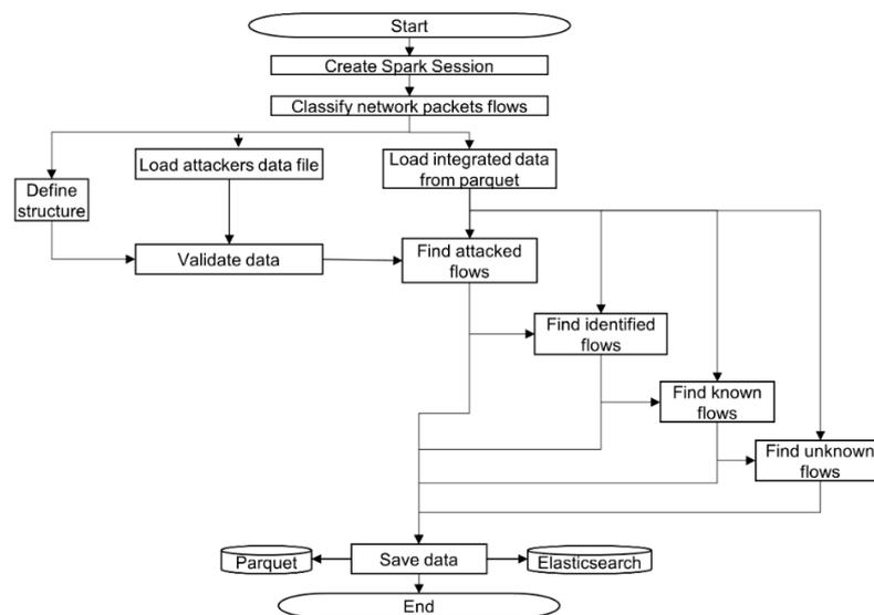
Figure 9. Design of network packets flow classification component.
