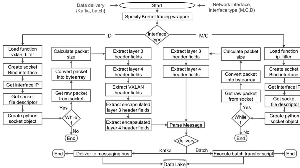
Figure 4. Design of network packets flow collection component.
