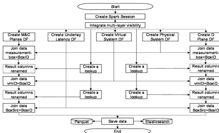
Figure 8. Design of multi-layer visibility data integration component.
