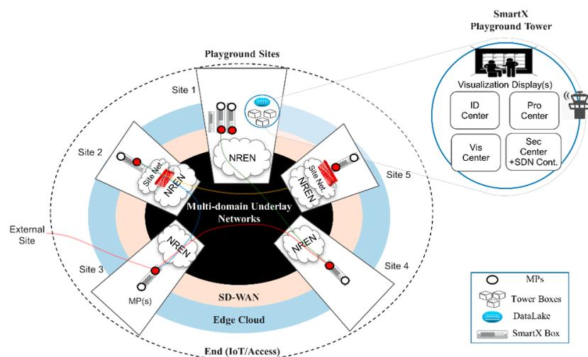
**Figure 1.** OF@TEIN playground as a software-defined networking (SDN)-enabled multisite cloud.
