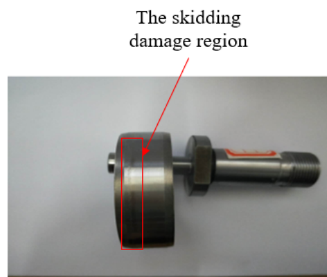
Figure 7. Tested roller and inner ring after skidding damage.
