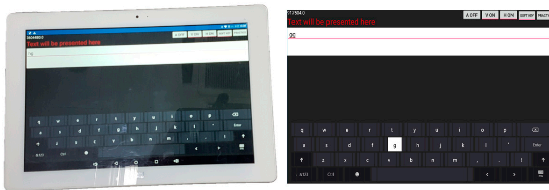
Figure 9. Soft keyboard design and a user interface implemented on the Android platform with a 10.1 inch commercial touchscreen (uPad) for a user study. The white text field was an area for a user to transcribe a red sentence randomly selected from a test set of sentences created by [23]. For the visual (V) condition, the pressed key was highlighted in white, while tactile key click feedback was additionally provided for the visual and haptic (VH) condition.
