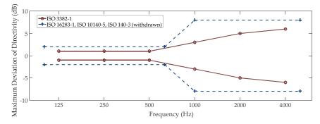
**Figure 1.** The maximum deviation of directivity of source in decibels for excitation with octave bands of pink noise and measured in free field for ISO 3382-1, ISO 16283-1, ISO 10140-5 and ISO 140-3 (withdrawn).
