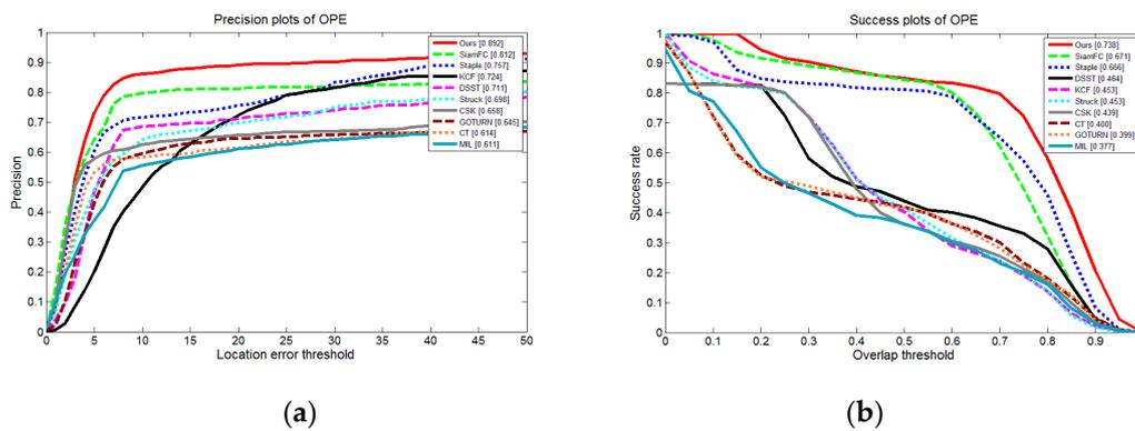
**Figure 10.** Results of different trackers on vehicle videos in OTB100: (a) one-pass evaluation (OPE) precision plots; (b) OPE success plots.
