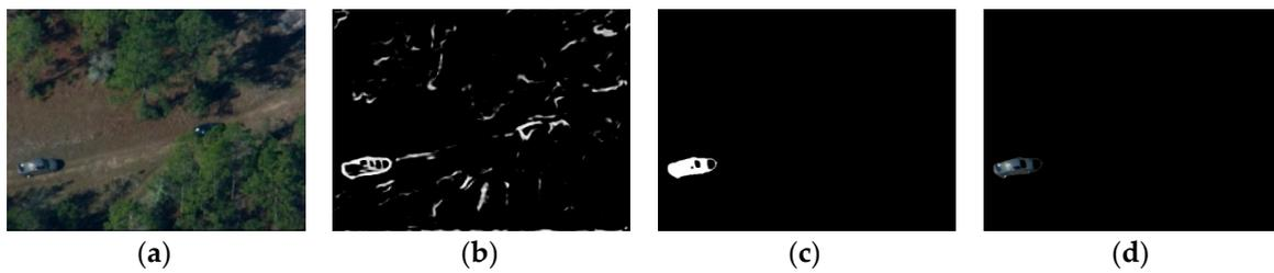
**Figure 5.** Shape-adaptive template generating process: (a) original image; (b) contour map; (c) target mask; (d) target template.
