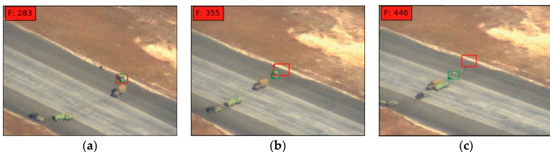
**Figure 1.** Example of false tracking due to target deformation: (a–c) are images to show tracking results for three frames in DARPA dataset, green boxes, ground truth; red, tracking results.
