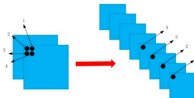
**Figure 6.** Passthrough-layer function: black circles with numbers indicate pixel in feature map before and after going through passthrough layer.
