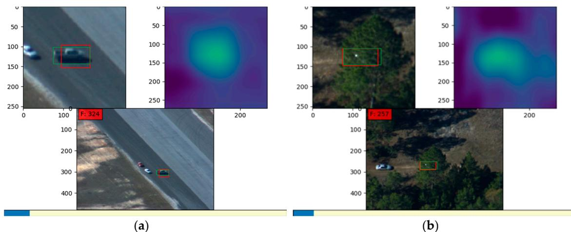
**Figure 7.** Results during (a) deformation and (b) occlusion. Bottom, tracking result in origin frame; top left, cropped image showing partial enlarged detail of tracking result; top right, corresponding heat map denoting similarity. Green boxes, ground truth; red, tracking results.
