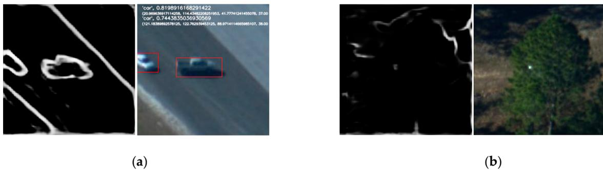
**Figure 8.** Outputs from template-update network under (a) deformation and (b) occlusion: left of each group, output from contour-detection network; right output from target-detection network.
