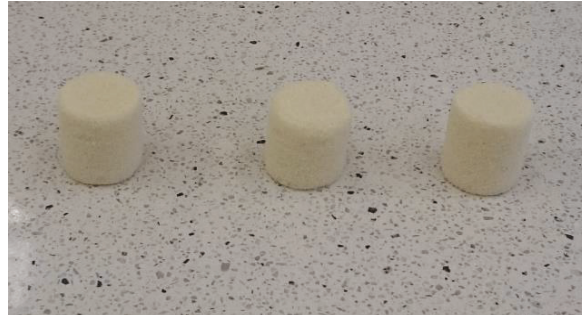
Figure 1. Samples made of polyurethane foam subjected to static compression.
