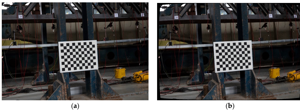
Figure 6. Camera calibration distortion adjustment; (a) original image; (b) image after distortion correction.
