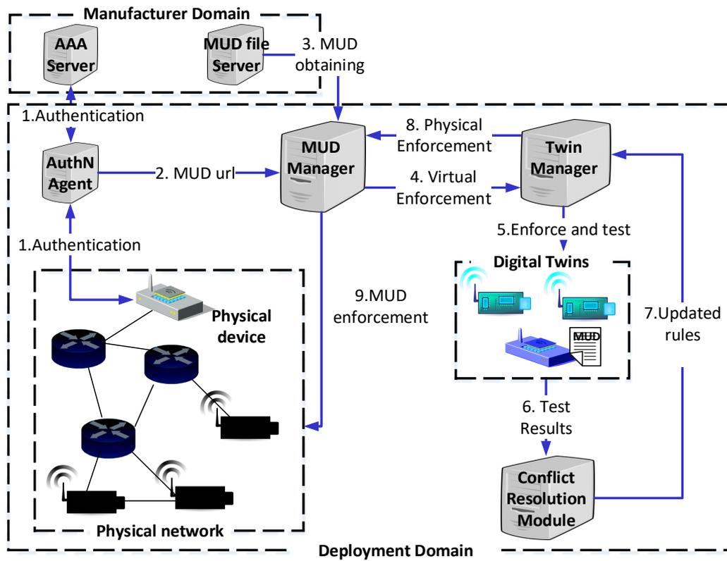
Figure 5. Integrating MUD-enhanced bootstrapping with digital twins.
