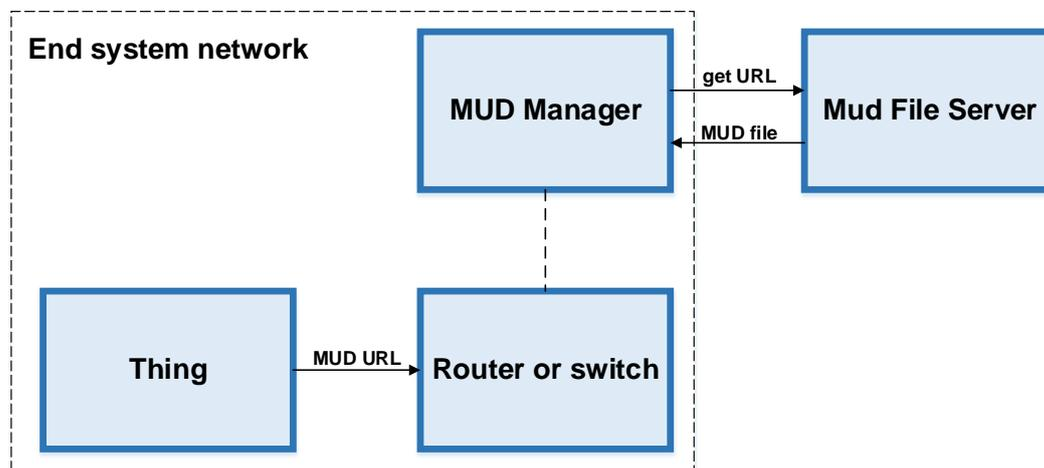
**Figure 1.** Manufacturer Usage Description architecture.
