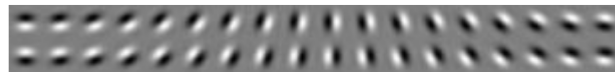
Figure 3. Filters for detecting edges. We use a bank of 2D Morlet wavelet kernels distributed in 36 orientations at 10° intervals.
