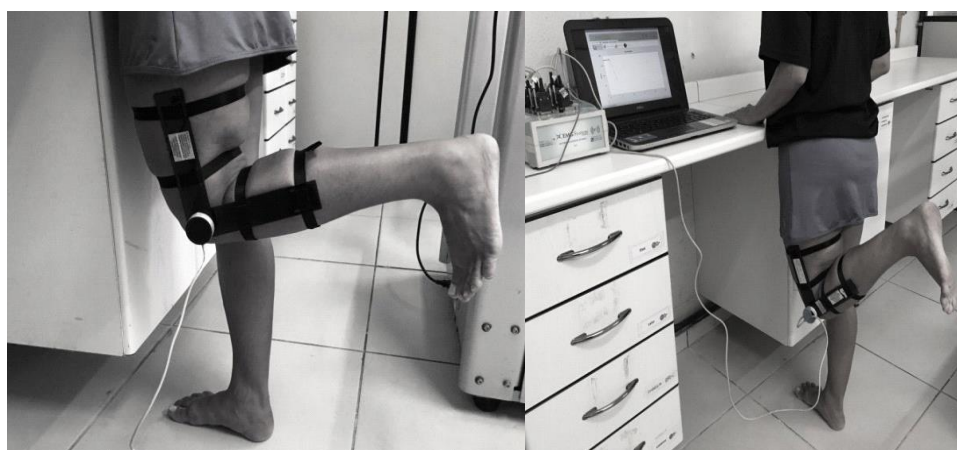
Figure 3. Position of the goniometer on the lower limb for measurement of knee range of motion (ROM).
