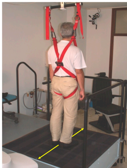
Figure 1. This shows a platform that can produce movements of the supporting base in various directions in the horizontal space according to different driving functions.
