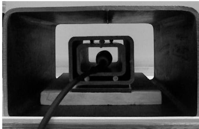
**Figure 1.** Three concentric steel shields providing a magnetic field attenuation of 144, with the Narda EFA-300’s magnetic field probe inserted at the culture position.
