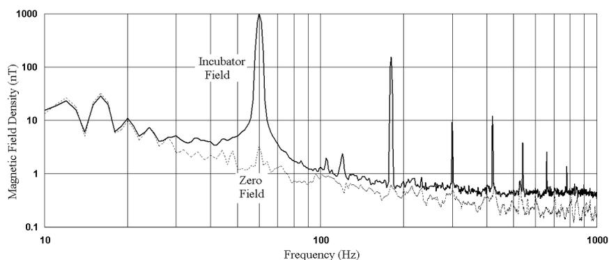
**Figure 2.** Spectral distribution of magnetic field density at “Incubator Field” and “Zero Field” positions. The 60-Hz component of “Incubator Field” corresponds to 1  $\mu\text{T}$ .
