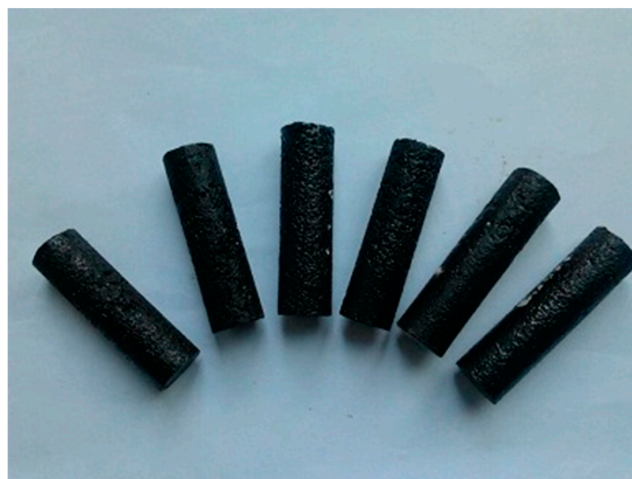
Figure 4. Fabricated asphalt mortar samples for dynamic modulus test.
