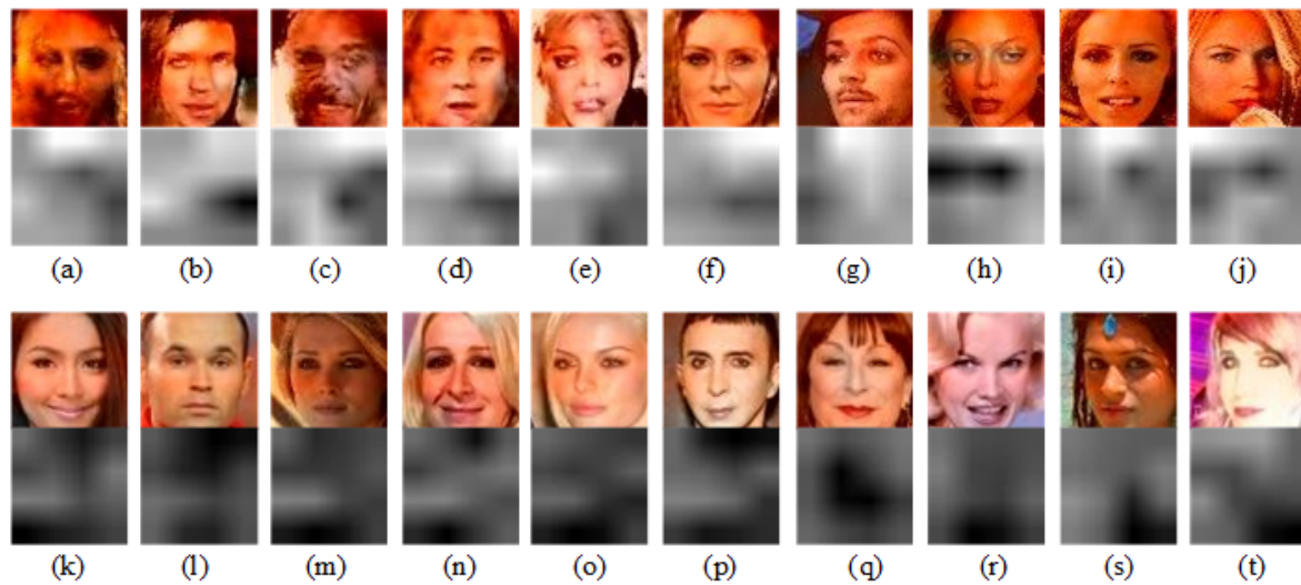
Figure 5. The visualized fake feature map for localization of fake regions in face images generated by the (a–e) WGAN [16] and (f–j) PGGAN [1]. (k–t) are the real images and the corresponding feature responses.
