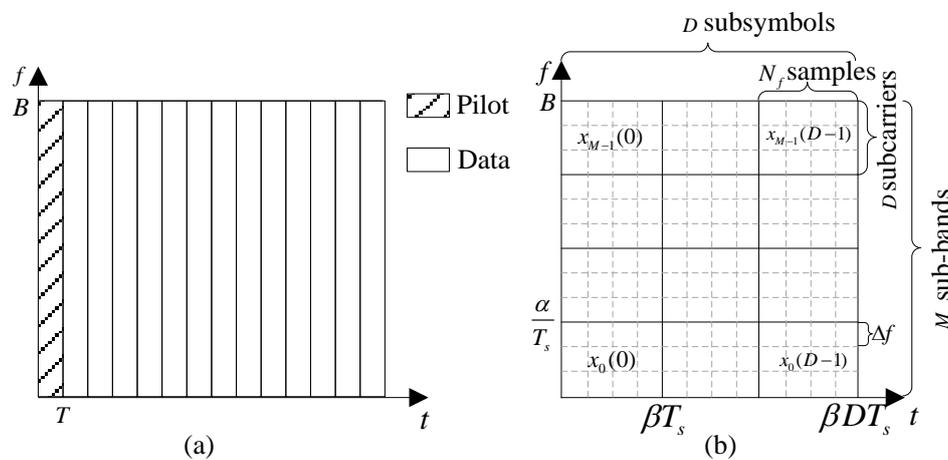
**Figure 3.** DBT-MC-FTN time-frequency resource block of one subframe: (a) DBT-MC-FTN transmission subframe structure; (b) the time-frequency grid of a DBT-MC-FTN symbol.
