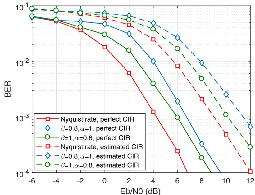
**Figure 7.** BER performance of DBT-MC-FTN and orthogonal symbols with perfect and estimated channel impulse responses (CIRs) over the TU-6 channel, where the parameters of the DBT-MC-FTN system were set to  $(\alpha, \beta)=(0.8, 1)$  and  $(1, 0.8)$ , and the number of iteration was set to 5. LS channel estimation with DFT interpolation method using DBT-MC-FTN pilots over the TU6 channel, and ZF channel equalization was utilized.
