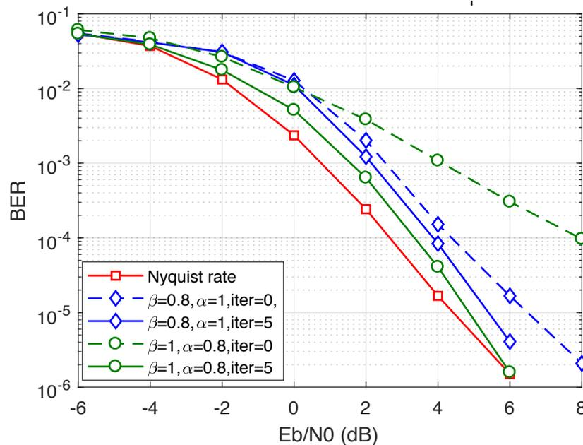
**Figure 6.** BER performance of DBT-MC-FTN and orthogonal symbols over the AWGN channel, where the parameters of the DBT-MC-FTN system were set to  $(\alpha, \beta)=(0.8, 1)$  and  $(1, 0.8)$ , and the number of iterations were set to 0 and 5.
