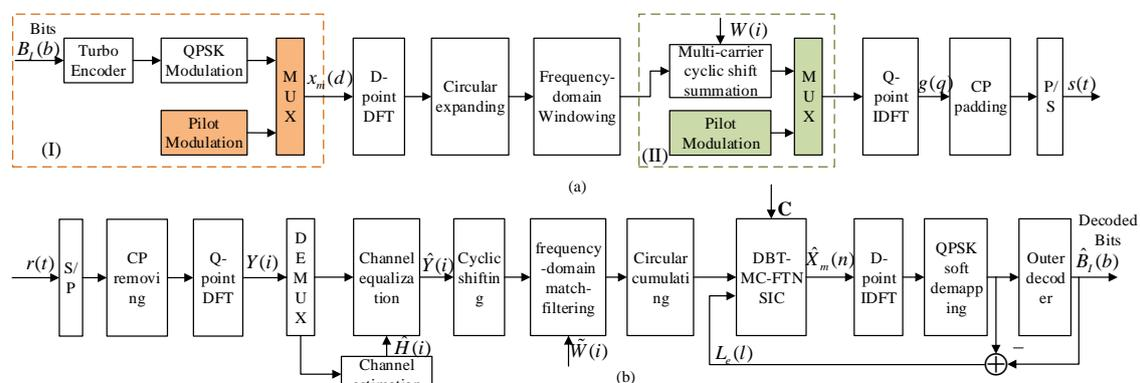
**Figure 1.** Block diagram of the DFT based block transmission for multicarrier faster-than-Nyquist (DBT-MC-FTN) transceiver: (a) transmitter: Scheme I: Channel estimation using DBT-MC-FTN pilots; Scheme II: Channel estimation using orthogonal pilots; (b) receiver.
