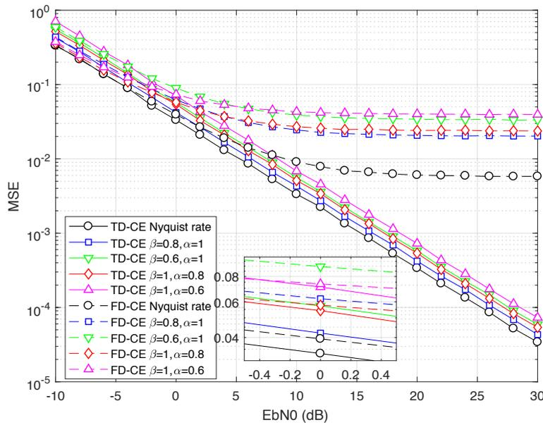
**Figure 4.** Mean squared error (MSE) performance of time-domain channel estimation (TD-CE) and frequency-domain channel estimation (FD-CE) methods using DBT-MC-FTN pilots over the TU-6 channel, where the parameters of the DBT-MC-FTN system were set to  $(\alpha, \beta)=(0.8, 1)$ ,  $(0.6, 1)$ ,  $(1, 0.8)$  and  $(1, 0.6)$ .
