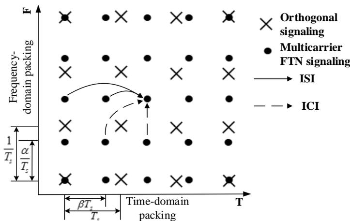
**Figure 2.** Illustration of the time-frequency grid of multicarrier FTN symbols and orthogonal symbols.
