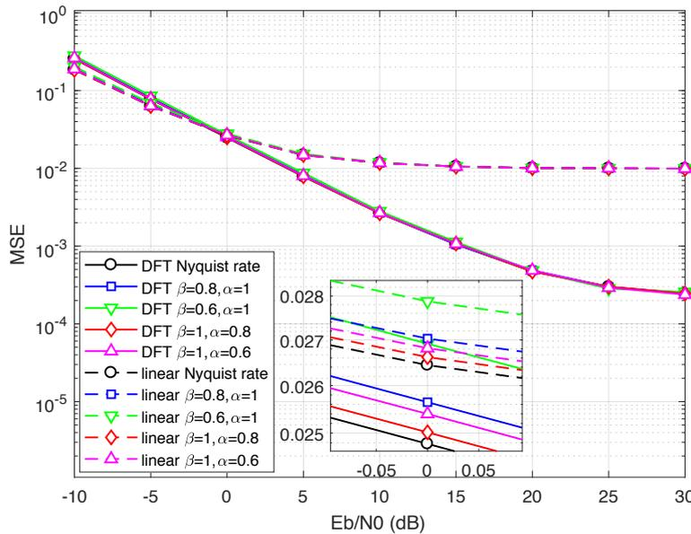
**Figure 5.** MSE performance of least square (LS) channel estimation with linear and DFT interpolation methods using orthogonal pilots over the TU-6 channel, where the parameters of the DBT-MC-FTN system were set to  $(\alpha, \beta)=(0.8, 1)$ ,  $(0.6, 1)$ ,  $(1, 0.8)$  and  $(1, 0.6)$ .
