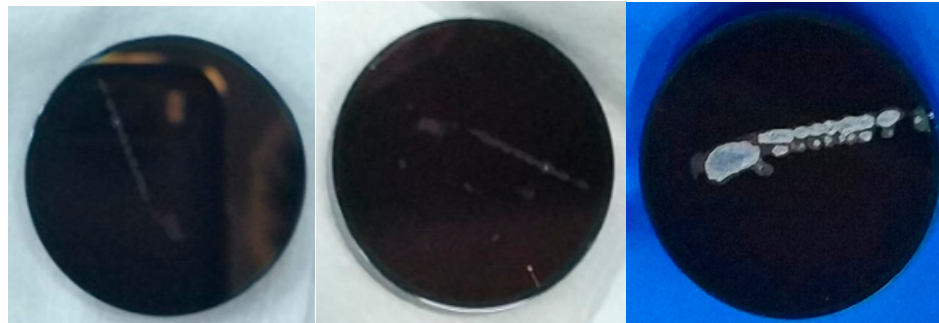
Figure 9. Damage phenomenon of the Ge window by the composite laser.
