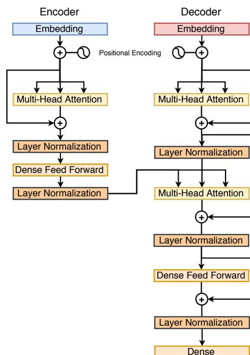
Figure 8. Transformer architecture overview.
