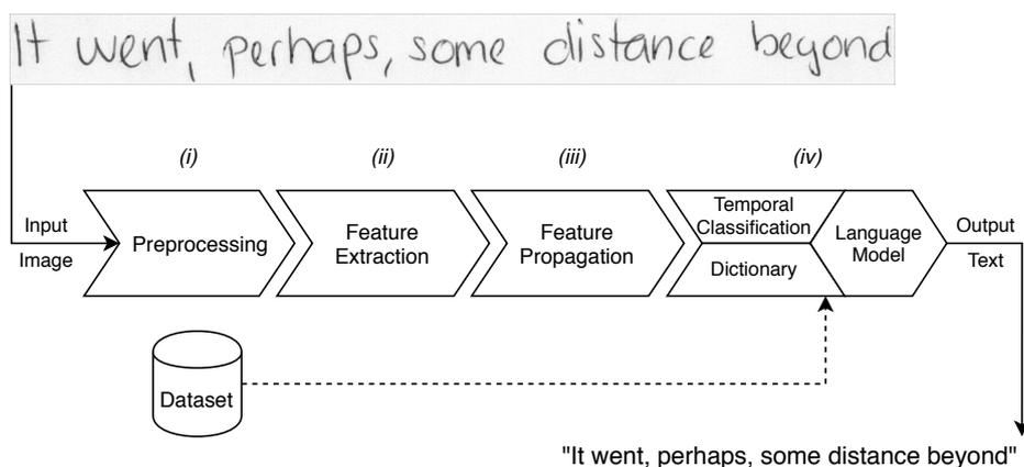
Figure 1. Workflow of the offline handwritten text recognition system.
