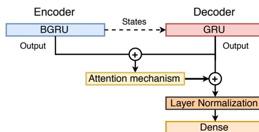
Figure 4. Proposed encoder–decoder architecture using Bidirectional Gated Recurrent Unit (BGRU) as encoder input and Gated Recurrent Unit (GRU) as decoder input.
