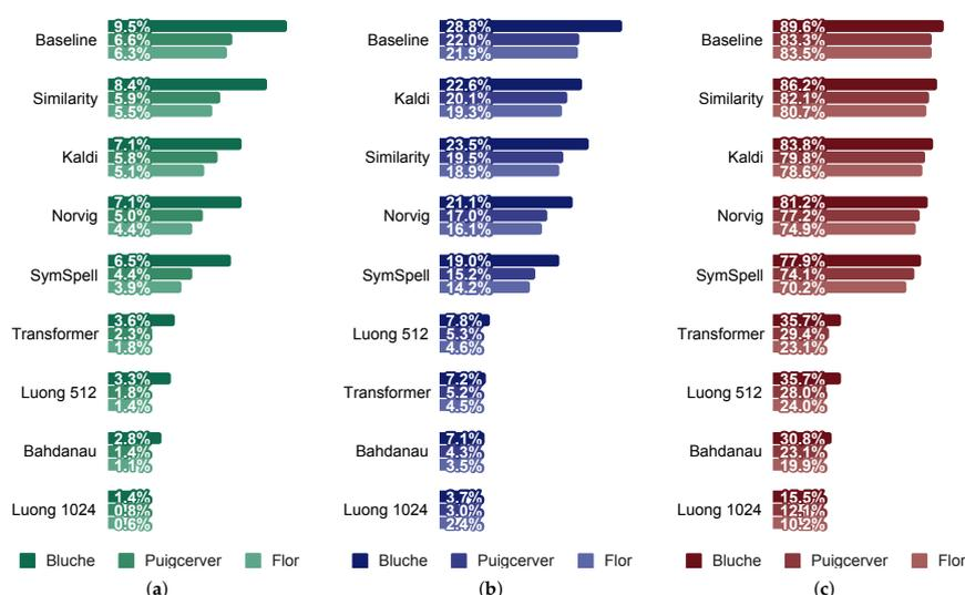
Figure 16. Error rates in the RIMES dataset (lower is better), (a) Character Error Rate (CER); (b) Word Error Rate (WER); (c) Sequence Error Rate (SER).
