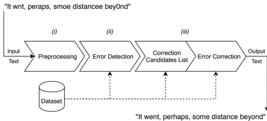
Figure 2. Workflow of the spelling correction system.
