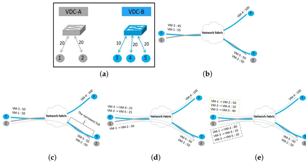
**Figure 6.** The bandwidth allocation mechanism. (a) The VN demands; (b) Initial allocation; (c) Rate stipulation (1 flow); (d) Rate stipulation (3 flows); (e) Dynamic flow rate adjustment.
