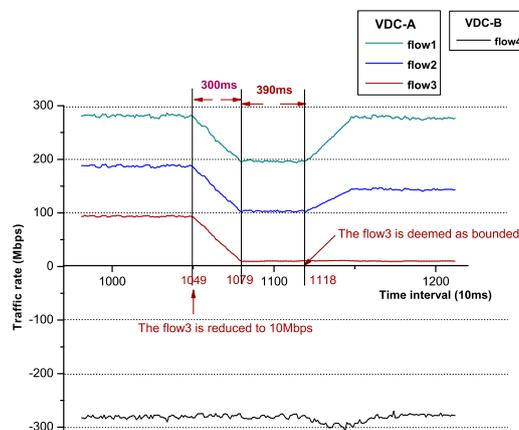
Figure 12. The detailed variation of flow rates in  $[t_0, t_1]$ .
