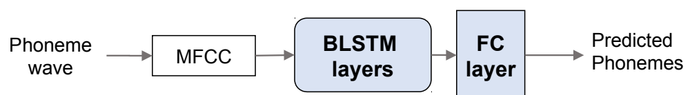
Figure 5. Phoneme classification model architecture for the baseline, as well as Vowel and Mixed groups.
