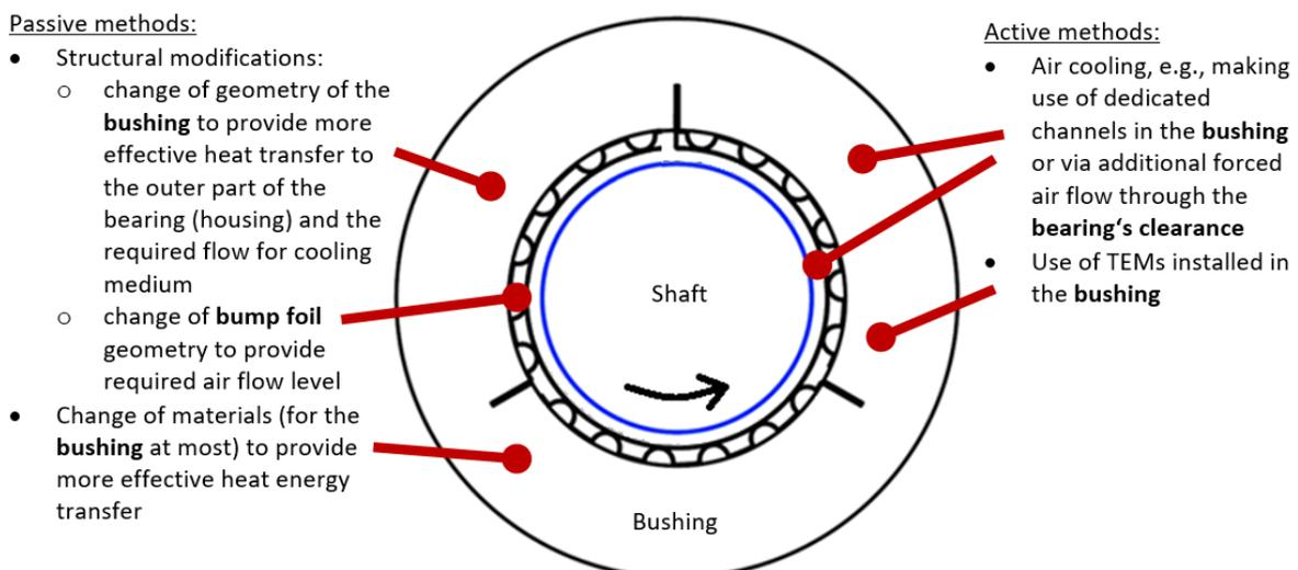
**Figure 3.** Thermal management in GFBs applied to enhance the performance of the bearings and prevent the loss of thermal stability. Heat energy source and sink components may be adequately installed to control the heat flow through the GFBs' body and prevent from undesirable excessive temperature gradients.
