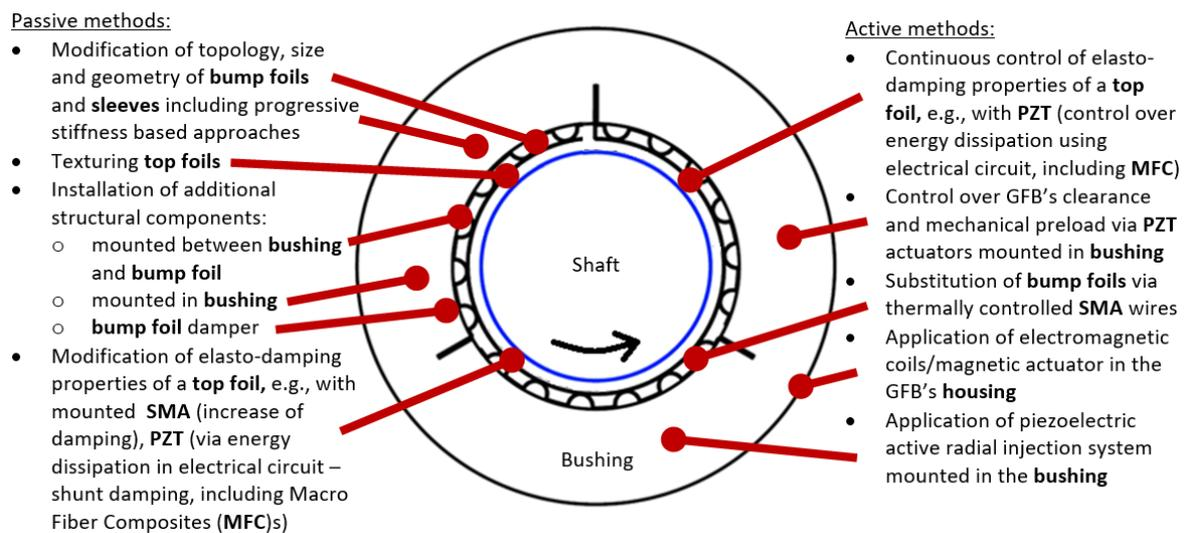
**Figure 2.** Scope of structural modifications in GFBs introduced to enhance the elasto-damping properties of the bearings. Various topology, size and geometric changes may be taken into account to improve the performance of GFBs. The modifications may affect both the bushing and specialized foils. Moreover, additional components (also made of smart materials) may be used to achieve an advantageous change in the bearing's properties.
